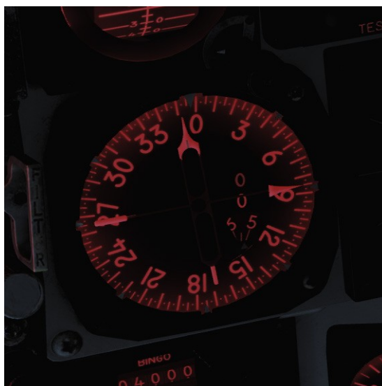
Figura 12: BDHI, Bearing Distance Heading Indicator
